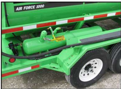
■ Emulsion Line Clean out
