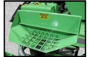
The hopper receives aggregate from the dump truck.
