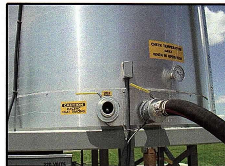
Heated & Insulated ball valves at the base of tank gravity feed emulsion to the Total Patcher.
